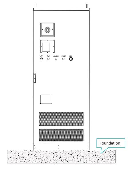
• The cabinet is fixed at the bottom, and holes should be pre-opened on the installation site in accordance with the fixed holes (marked in red) in the base of the cabinet. See the drawing below.
