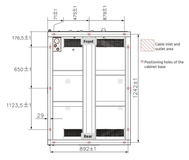
Positioning holes of the cabinet base (Unit: mm)
