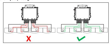
Step 8. Connect APsystems Microinverters to Grid
