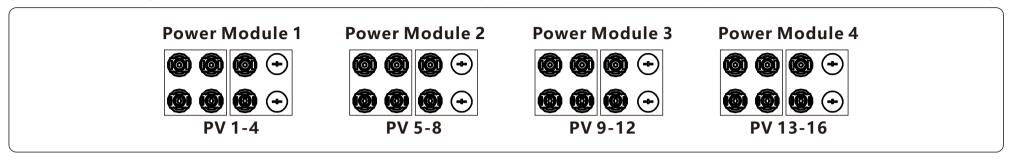
If four power modules are indeed required to connect the solar panels unevenly, for a power module which is connected to three strings, it is necessary to ensure that the power of each PV strings connected under this power module does not exceed 11.3kW to achieve better power generation performance. In the case that the power difference between each PV string is less than 10%, the 3 common cases are showing below.
