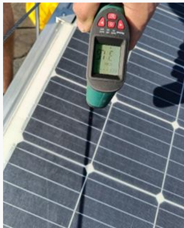
Figure 3: Temperature measurement of a section of a PV cell in the shadow, with infrared laser thermometer
