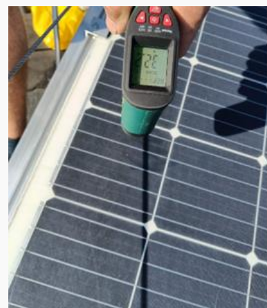
Figure 4: Temperature measurement of a section of a PV cell in the sun, with an infrared laser thermometer
