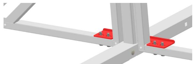
Place the **second** center bracket on top of the first bracket
