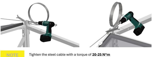
Tighten the steel cable with a torque of 20-25 N\*m
