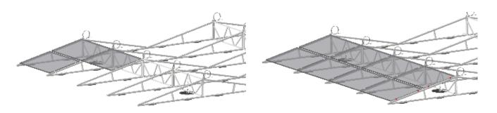
Follow the placement sequence of the panels as depicted below. The next step is the tensioning of the steel cable between the sides. Tighten the steel cable using the extended 13 mm socket (Article number 20-060-0033) with a torque of 20-25 N\*m. To prevent the steel cable from spinning while tightening, use the provided wrench (Article Number 20-060-0034) or a plier. To prevent friction welding of the stainless-steel nut and threaded end, lubricate the connection and tighten gently.
