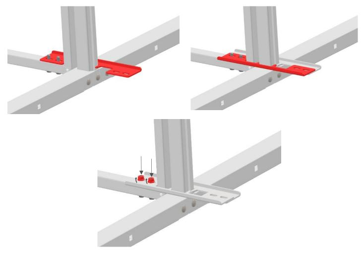
Use the two M8x16 mm allen bolt on the top of the side and the separately provided M8 flange nuts to attach the outside section of the center brackets.
