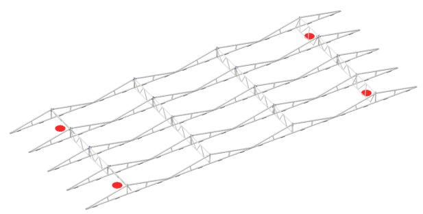
To easily install the roof anchors, it is possible to tilt the center in such a manner it doesn't obstruct the installation of the roof anchors. Tilt the centers at the locations of the anchors and mount the anchors.
