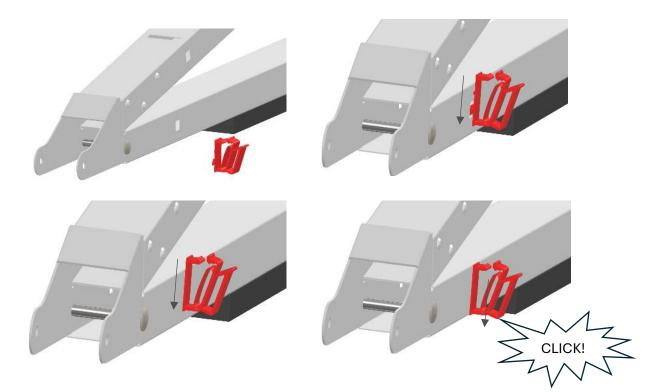
Cable management clips can be placed on either lower or upper part of the side as depicted in the drawing below.
