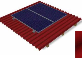
**Roof:** Fibre cement corrugated sheets with wooden purling **System:** Universal adapter Uno M10 / M12 with hanger bolt.
